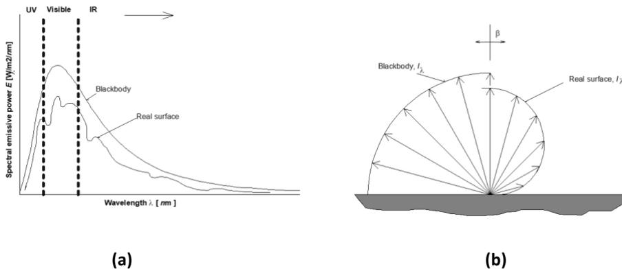
**Figure 1 - Comparison of blackbody and real surface emissions. (a) Spectral distribution, (b) Directional distribution ( $I_\lambda$  = radiation intensity,  $\beta$  = radiation angle) (Incropera & DeWitt, 1996)**
