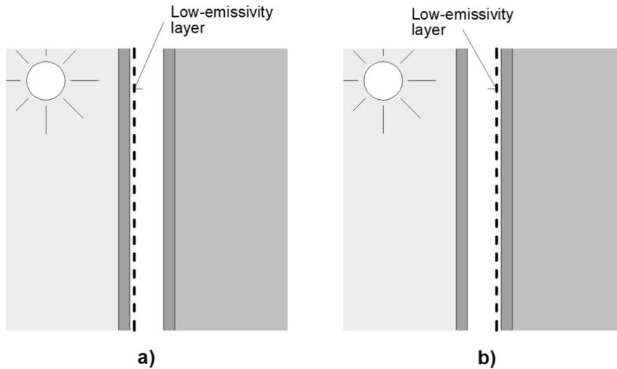
Figure 2 - Typical position of low-emissivity layer in double glazing. (a) High performance system, (b) Low-e system
