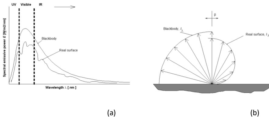
Fig. 1: Comparison of blackbody and real surface emissions. (a) Spectral distribution, (b) Directional distribution ( $I_\lambda$  = radiation intensity,  $\beta$  = radiation angle) (Incropera & DeWitt, 1996)
