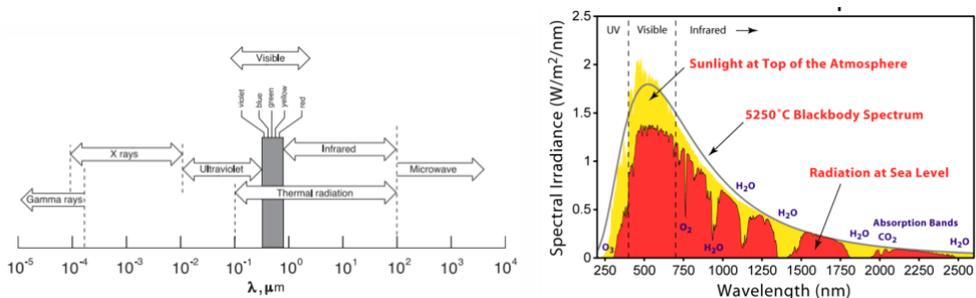
Fig. X Electromagnetic spectrum and solar radiation spectrum
