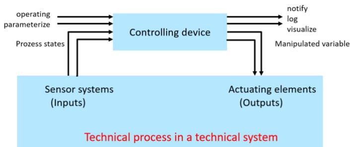
In order to automate a technical process, it is necessary both to obtain information about the process and to be able to actively interfere in the process. This process information is recorded
