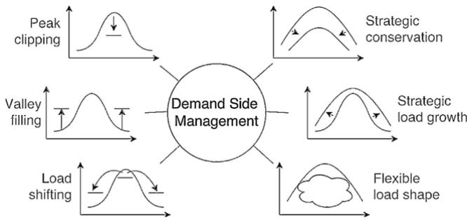
decreasing the energy consumption in general, Flexible Load Shape is used for modifying the energy needs of consumers according to the available energy. Peak Clipping is used for decreasing the energy consumption during the
