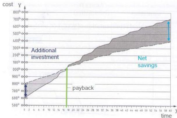
Figure 6.2.8 – Graphical reporting of whole-building level comparison accord. To ISO 15686-5:2017
