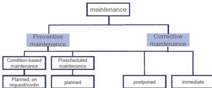
Figure 6.2.11 -Types of maintenance according to EN 13306:2017
