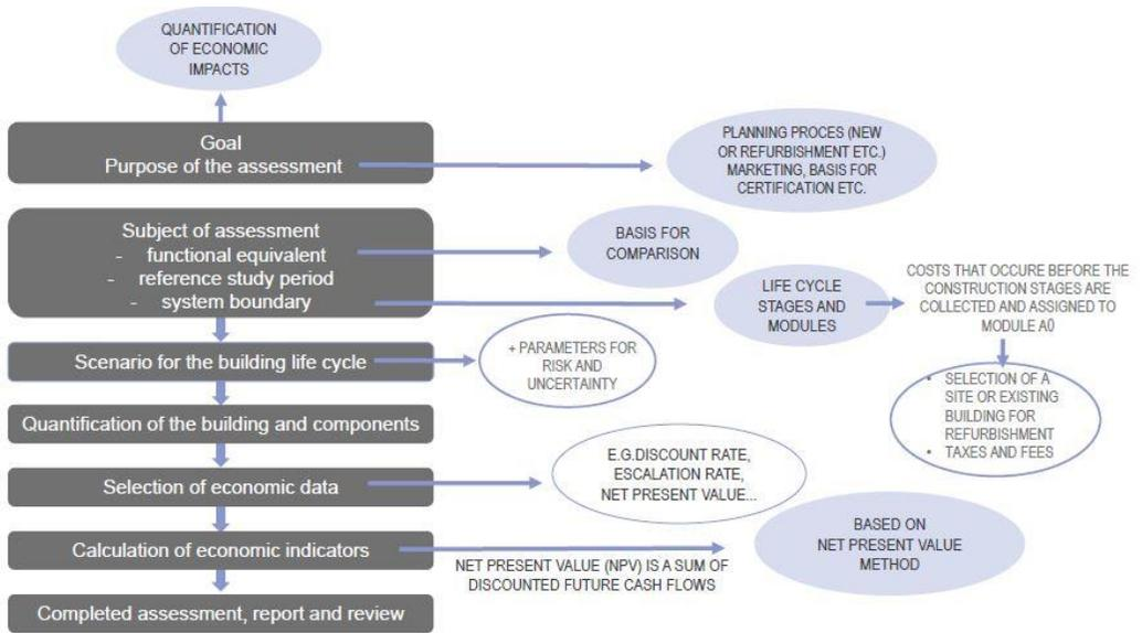
Figure 6.2.7 – simplified assessment steps for LCCA of buildings according to EN 16627
