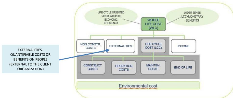
Figure 6.2.4 – LCC and WLC elements according to ISO 15686-5
