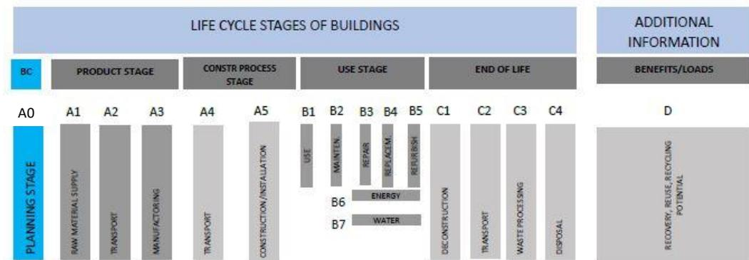
Figure 6.2.9 – Life cycle stages and system boundaries of LCCA. BC- before construction/pre construction.
