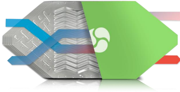
Figure 3.6.9. Operation of a plate heat exchanger
