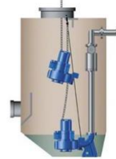
Waste water pump: Submersible motor pump with guide wire arrangement
